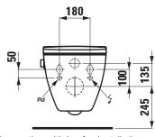
Connection with Laufen installation system LIS CW2
